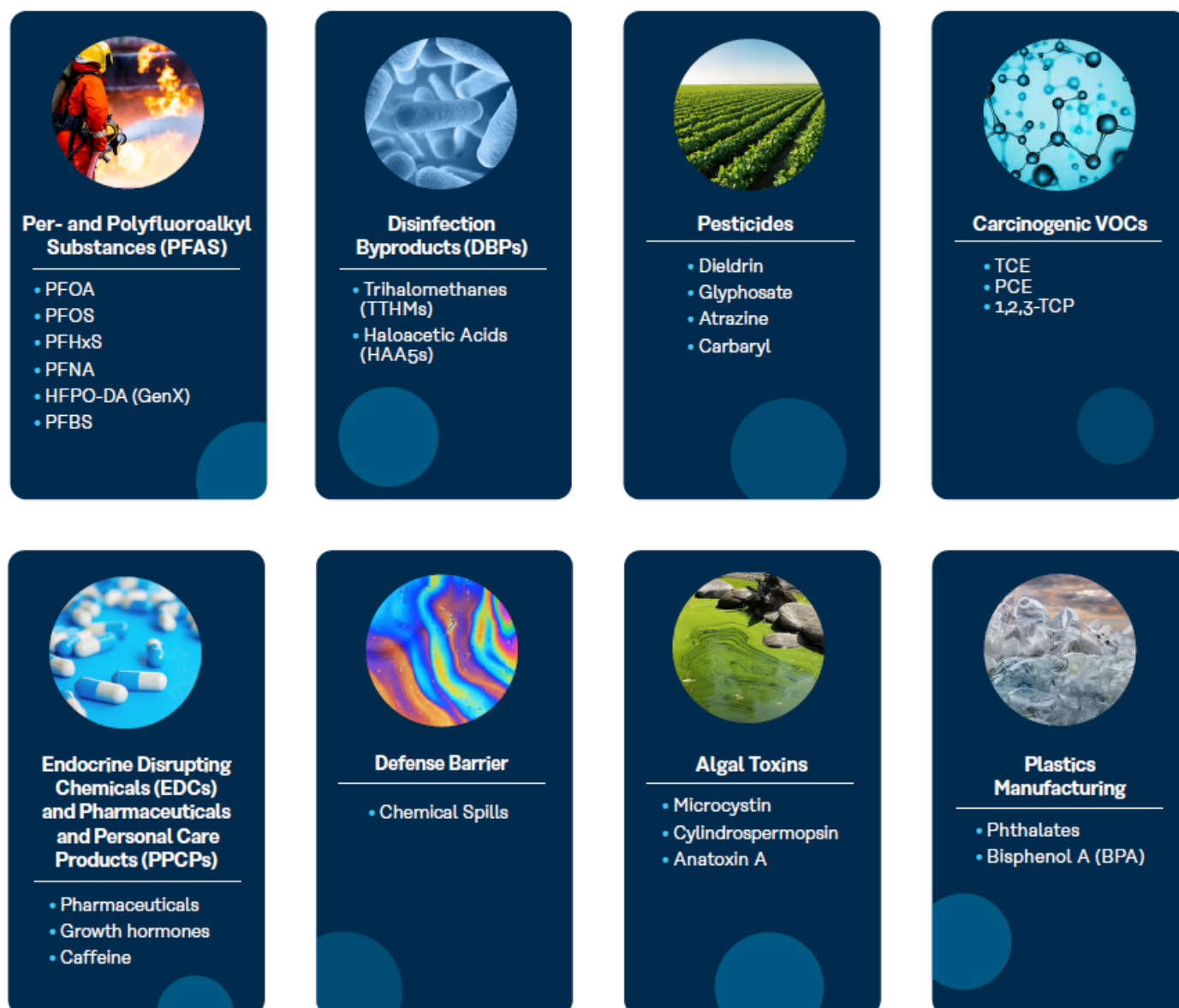
Figure 1. Activated Carbon Adsorption: Simultaneous Removal of Multiple Organic Contaminants in Water: GAC is an EPA-recognized best available technology (BAT) for removing an array of drinking water contaminants including PFAS, TOC, DBPs, VOCs, and 1,2,3-TCP, among others.
